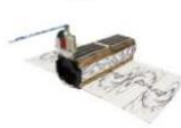
PlanetScope (Dove) Launch Mass 4kg
